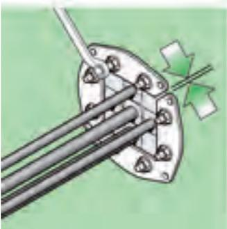
**7** Slide the two front plates together and tighten the nuts 2mm each time, applying equal pressure to both plates\*. The bolts should be tightened until the cables/pipes are sealed. A minimum of 10mm of thread should protrude on each bolt.
