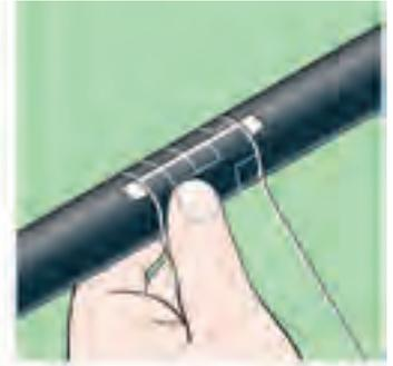
Hawke Cable/Pipe/Block Selection Gauge
